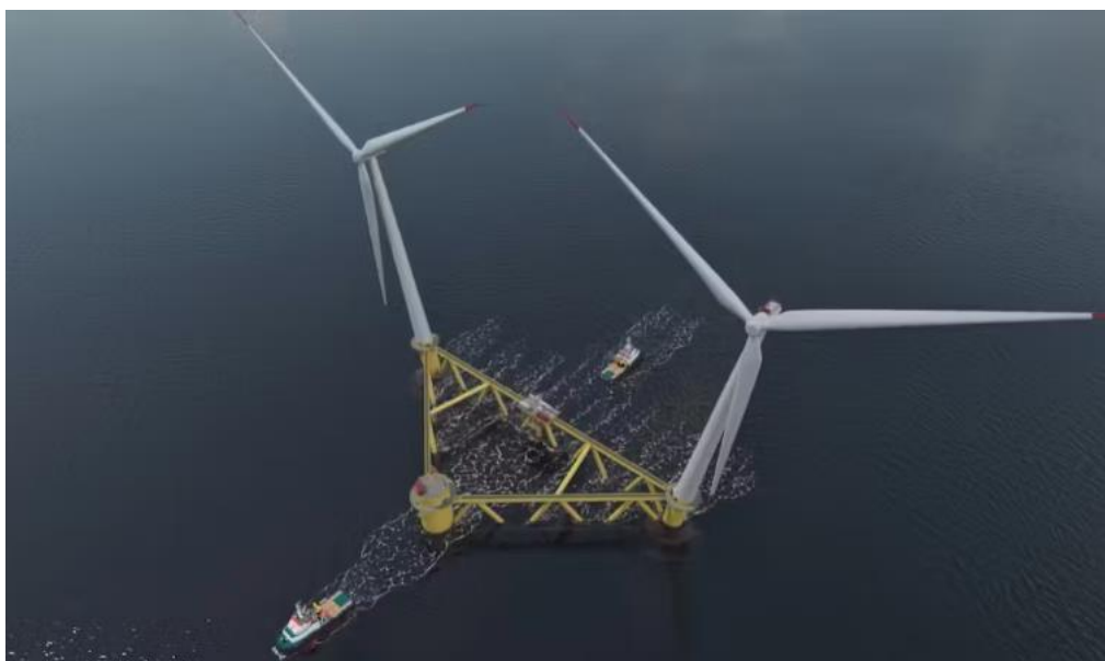
Figure 40 Hexicon AB TwinHub Platform [193]
